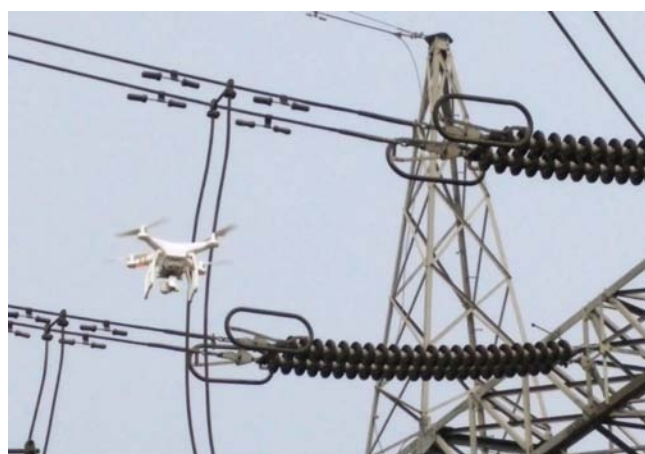
Aerial view of Transmission line patrolling through Drone
