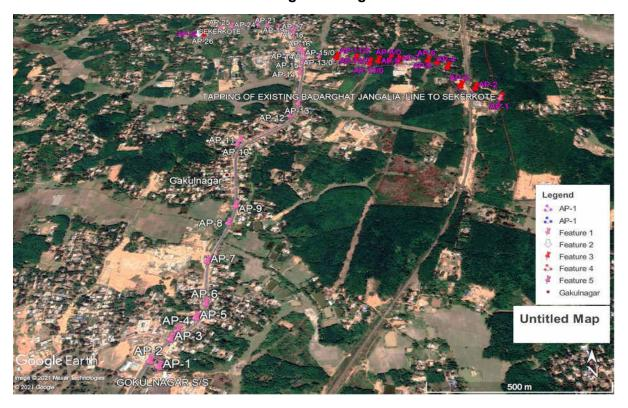
Route alignment of 33kV S/c line from 132/33kV Gokulnagar to 33/11kV Sekerkote substation
