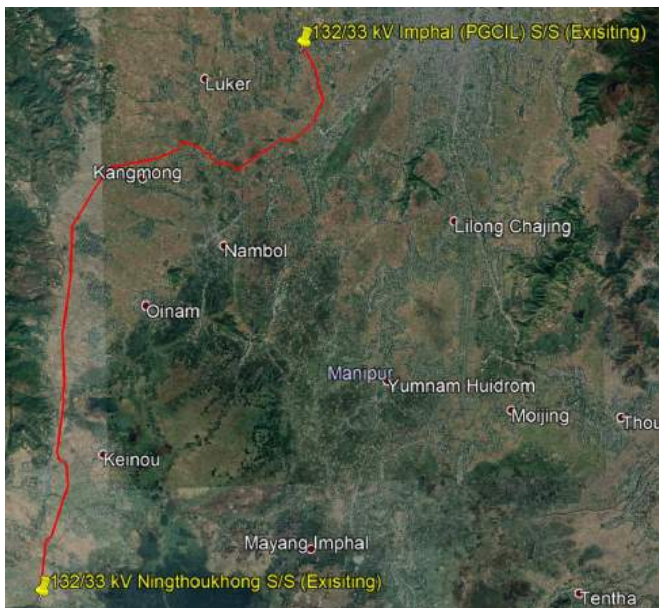
Figure 4.1: Satellite Imagery Showing Route of Imphal (PG) – Ningthoukhong 132 kV D/C Transmission Line
