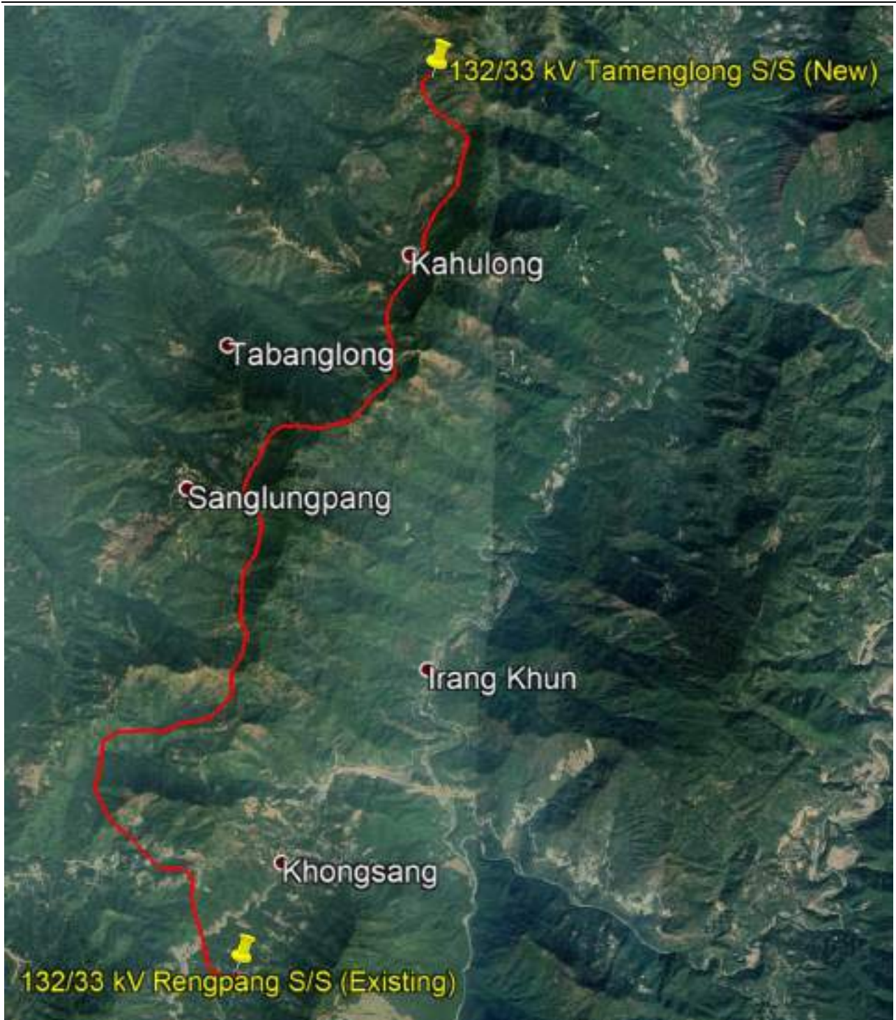
Figure 4.1: Satellite Imagery Showing Route of 132 kV S/C (on D/C tower) Rengpang – Tamenglong Transmission Line
