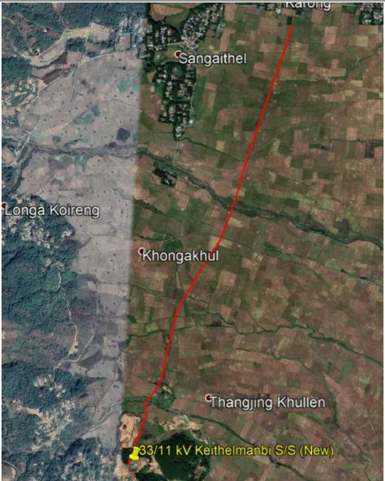
Figure 4.2: Satellite Imagery Showing Route of LIL of Yurembam Noney Line at Keithelmanbi
