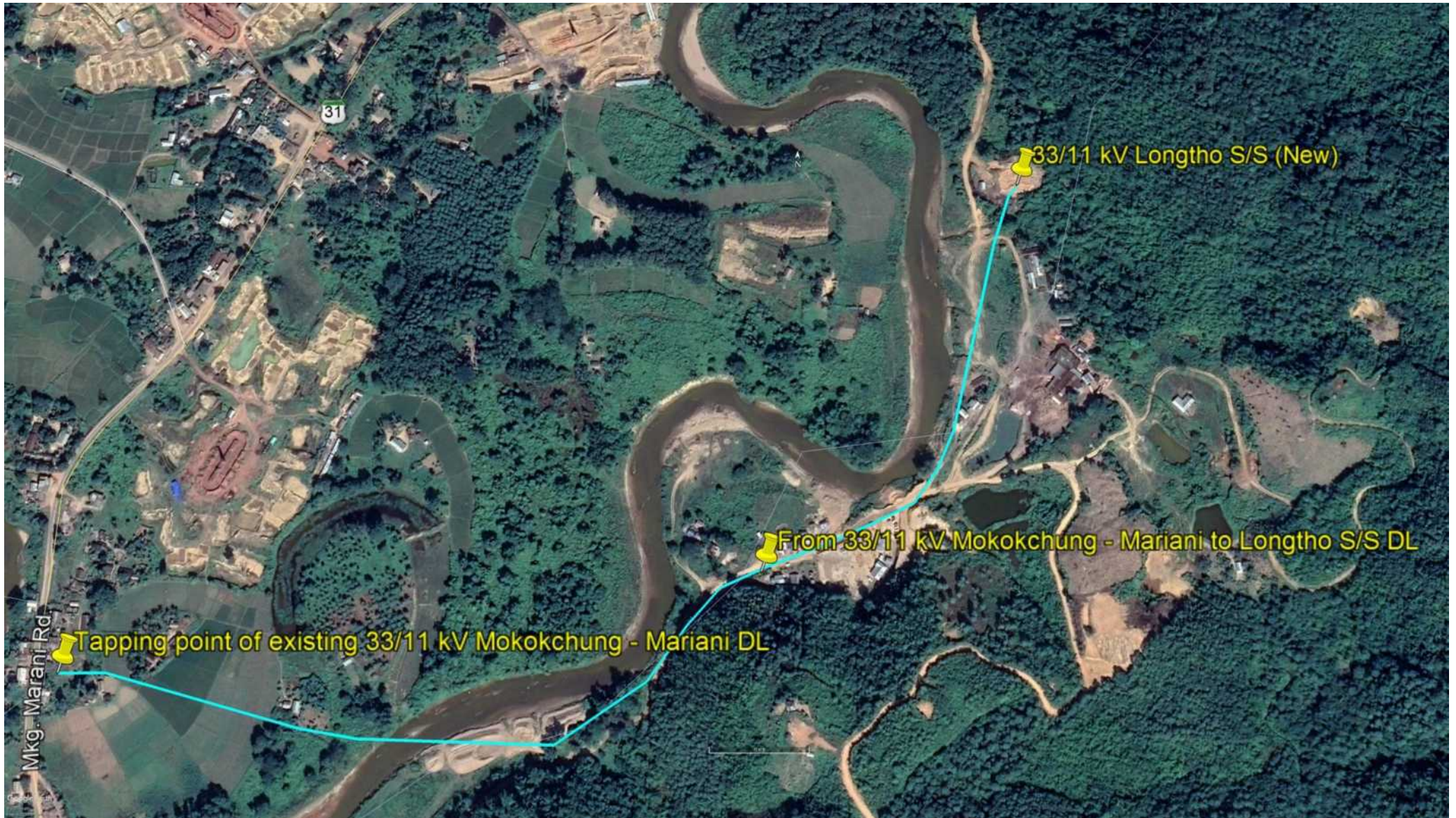
Figure 4.7: Satellite Imagery Showing Route of Existing 33 kV Mokokchung - Mariani Line to Proposed 33/11 kV Longtho S/s Distribution Line
