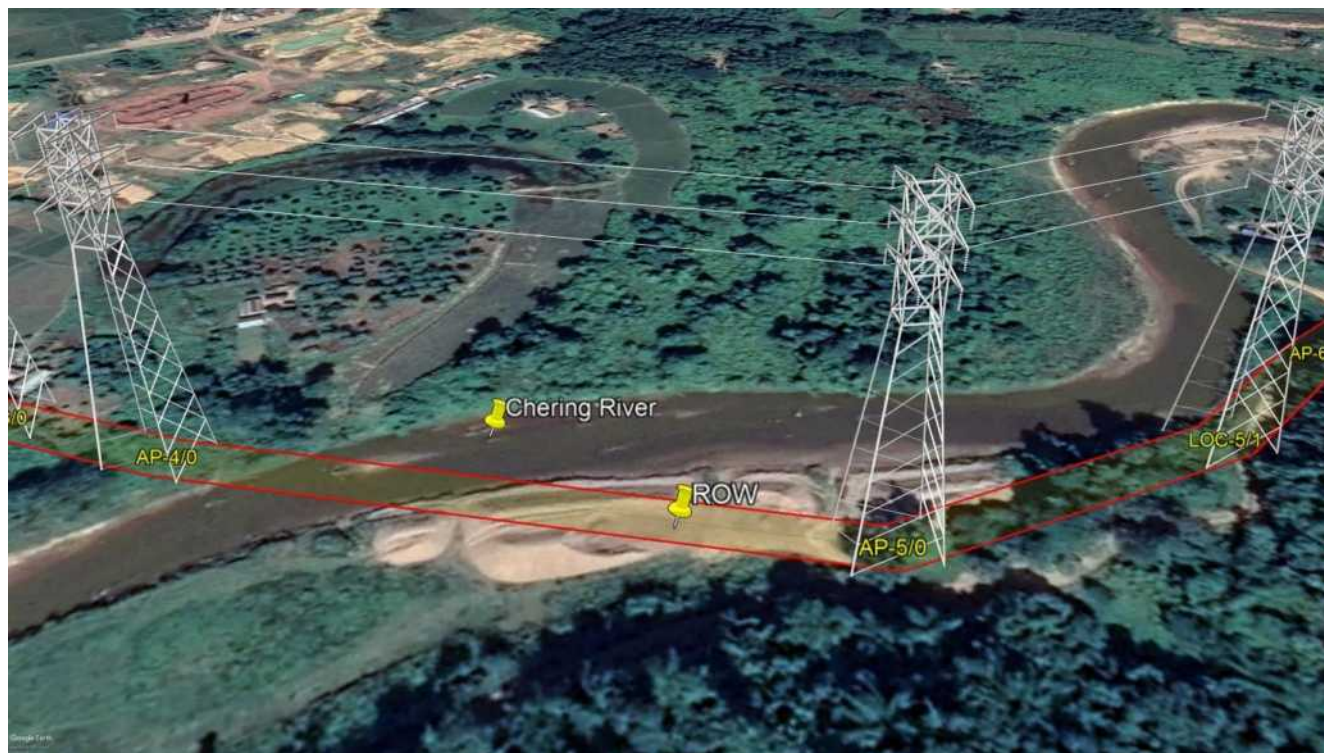
Figure 4.22: Increase in Length of Span Between Pole 4 and Pole 5 over Chering River
