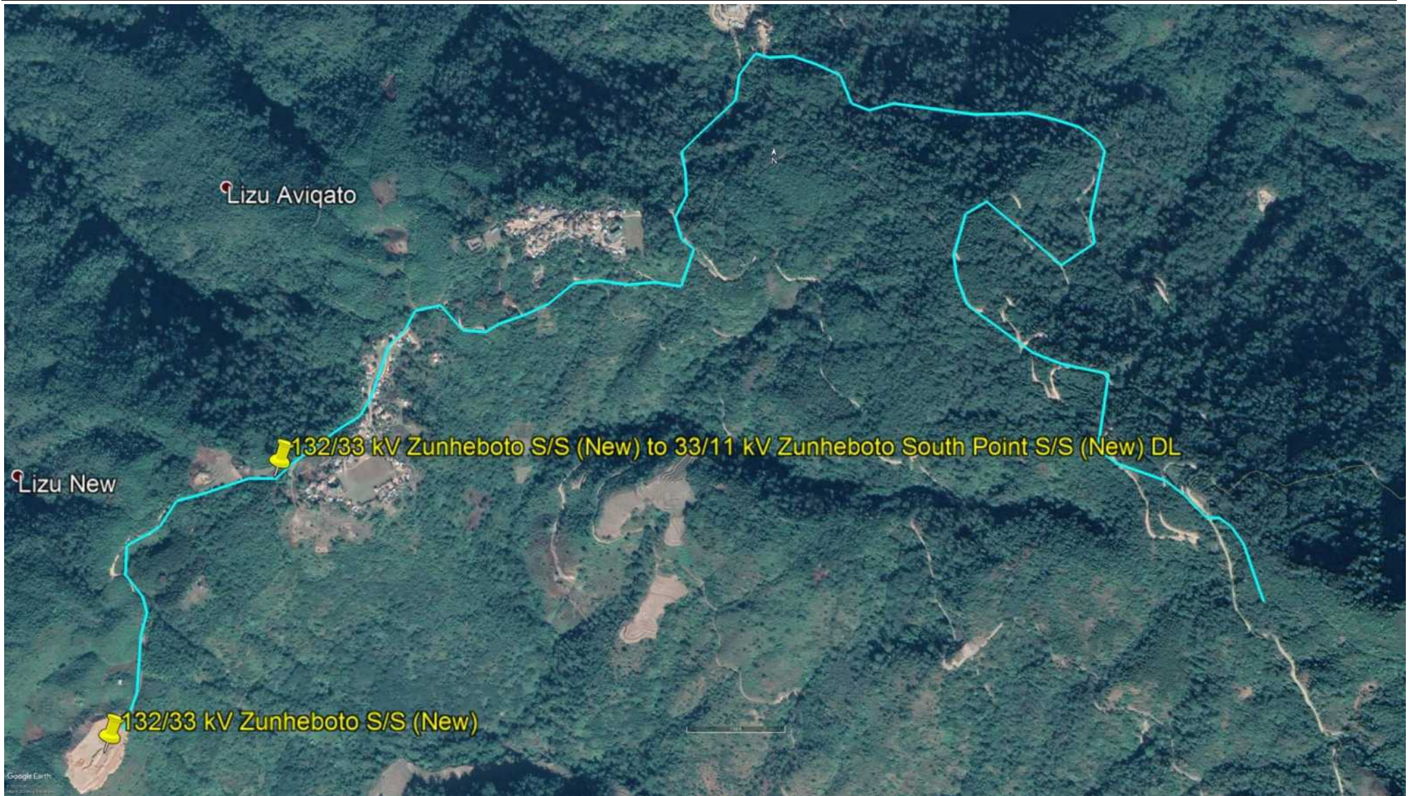
Figure 4.8: Satellite Imagery Showing Route of New 132/33kV Zunheboto S/S to New 33/11kV S/S Zunheboto South Point Distribution Line
