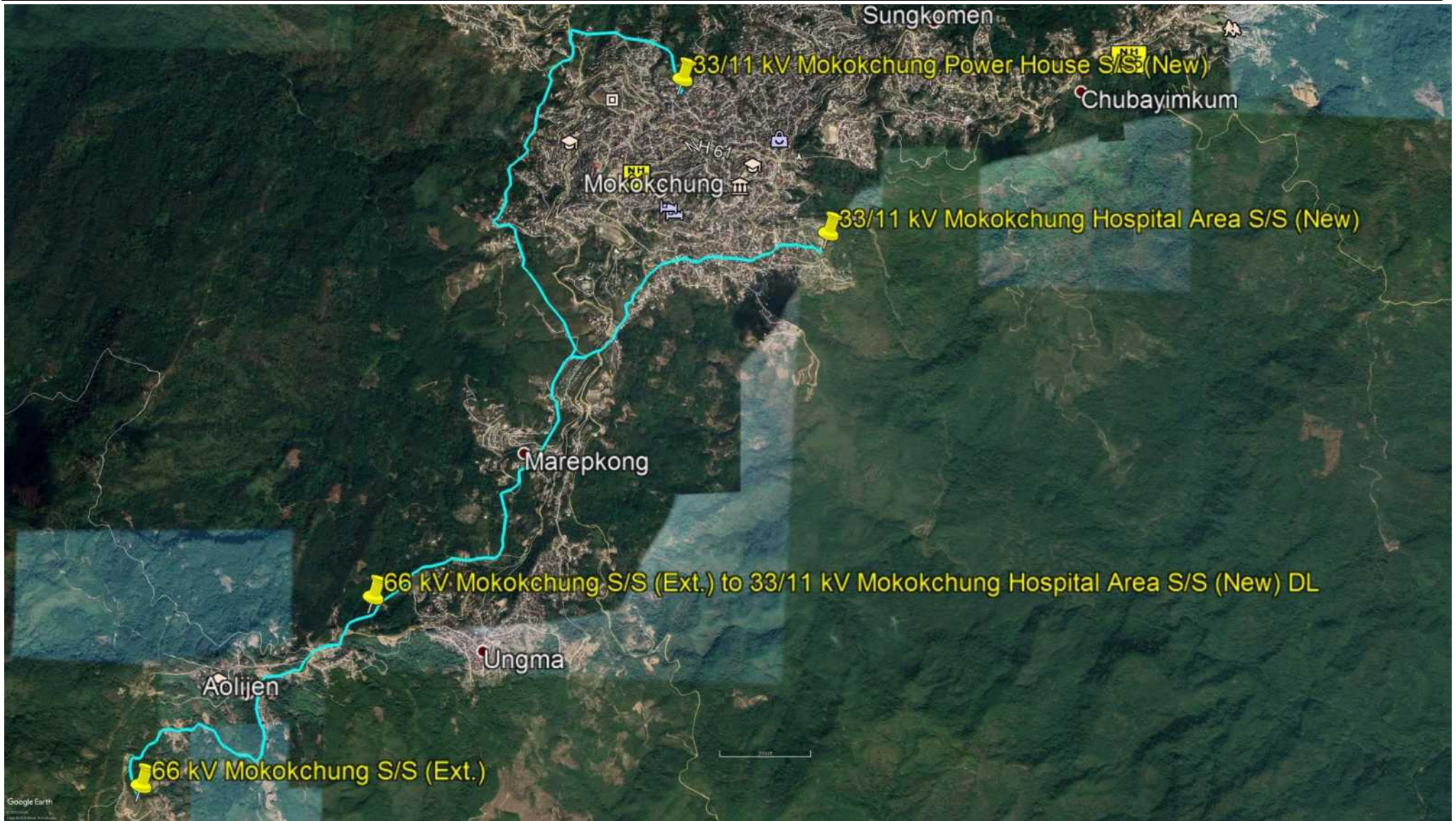
Figure 4.9: Satellite Imagery Showing Route of Existing 66/33kV Mokokchung S/S to New 33/11kV S/S Mokokchung Town Power House and Existing 66/33kV Mokokchung S/S to New 33/11kV S/S Mokokchung Town Hospital Area Distribution Lines
