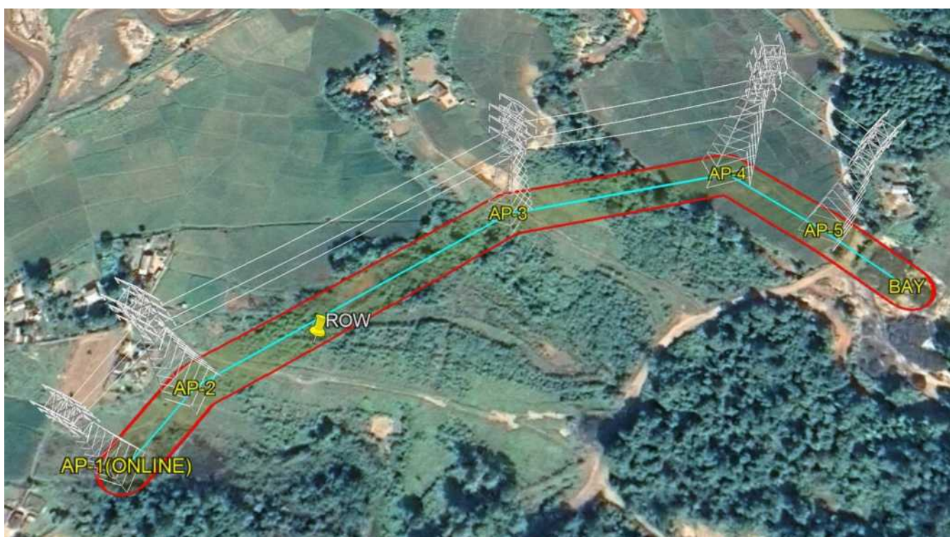
Figure 4.14: Major Features en route of LILO of 132kV S/C Mokokchung-Mariani at Longnak
