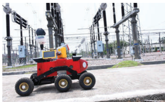
Substation Inspection Robot in switchyard
