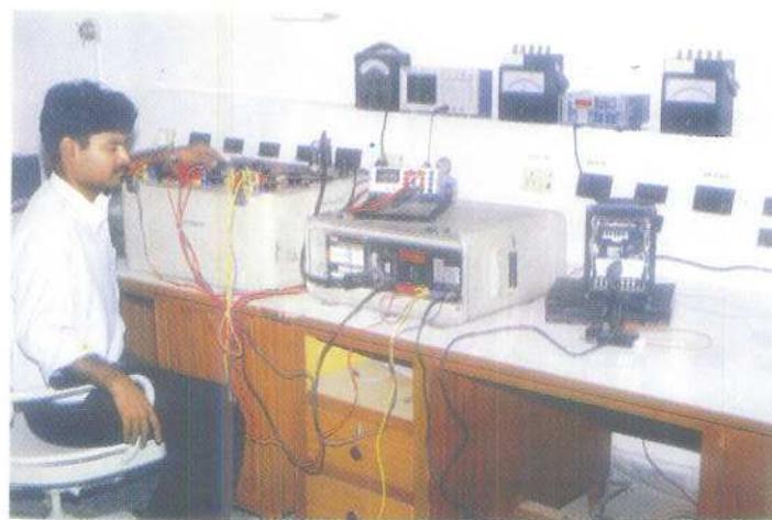
Energy Meter calibration being carried out by RTL Engineer
